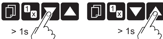
Fig. 24: Switching gauges on and off
