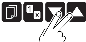
Fig. 32: Load factory settings: Press the arrow keys simultaneously > 2 seconds
