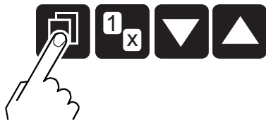
Fig. 27: Change from measuring mode to parameter mode
